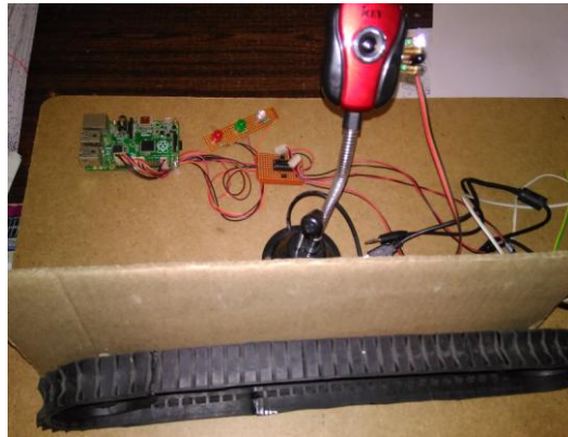
12) Conveyor belt, Raspberry pi and camera interfaced together
